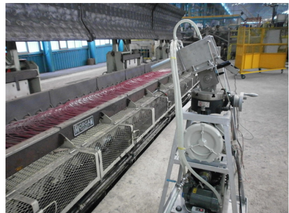
Fig.7(a). The wire rod temperature measurement for a fast air-cooling process (W/O Encopanel).
