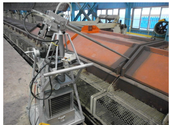
Fig.7(b). The wire rod temperature measurement for a slow air-cooling process (W/ Encopanel).
